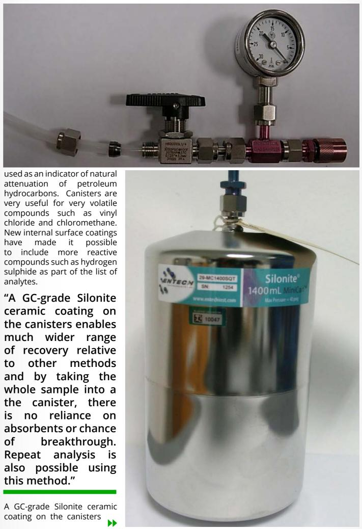
enables a much wider range of recovery relative to other methods and by taking the whole sample into the canister, there is no reliance **for** on absorbents or chance of breakthrough. Repeat analysis is also possible using this method.
