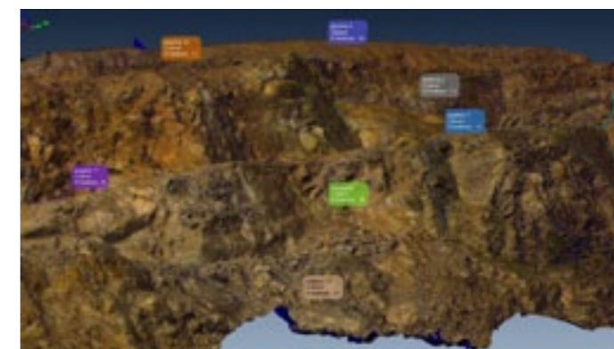
Figure 3 – Geological features (joints) digitised from “point-cloud”
