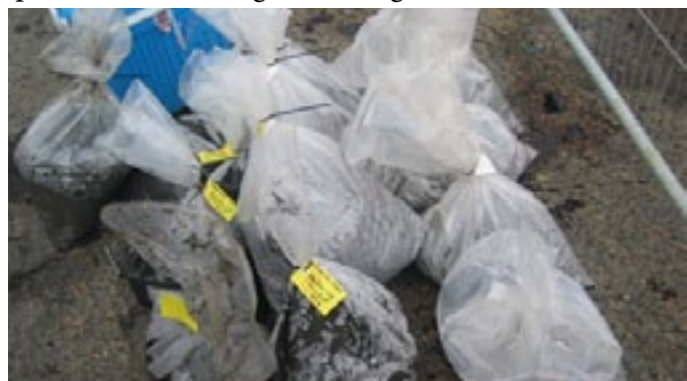
Bulk sample cannot be adequately sealed to allow an accurate determination of the moisture content.
