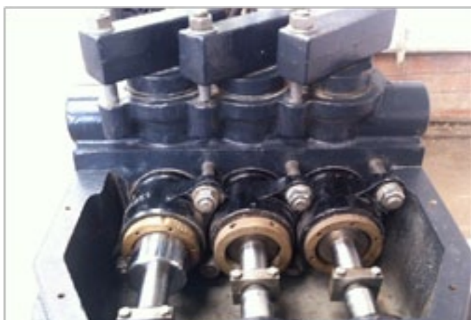
Ultra-Flow high pressure, high flow rate triplex mud pump for optimum drilling rates.
