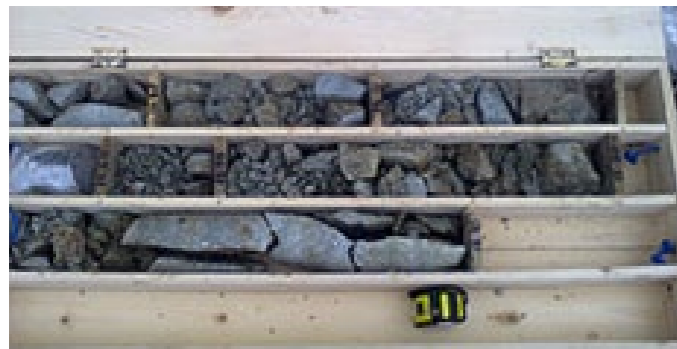
3. Proof that core can be recovered in poor ground conditions with expert advice.
