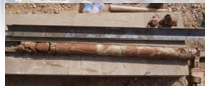
3. Good quality core recovered after Drilling Specialist made the Contractor unseize the core barrel
