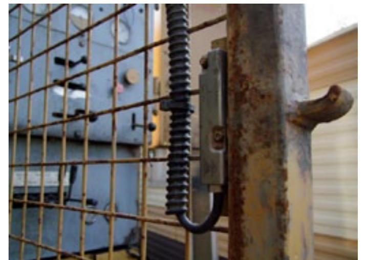
Industry endorsed: coded magnet interlock-switch.
