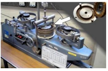
Aside from large research apparatus, the ringshear test is generally performed on an annulus 100 mm outer diameter, 70 mm inner, and 5 mm deep, which has been filled with remoulded fine grained soil.
