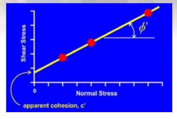
These parameters can be used in a variety of situations such as investigating slope stability, designing foundations and calculating lateral stresses on retaining walls. This gives rise to our first 'catch point':
