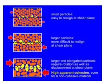
The larger and more angular the particles, the more force is required to move them, and the greater the shear stress that is developed. This is why the cohesion is reported as apparent cohesion: a non-cohesive material won't bind together, but the result may appear to show cohesion:
