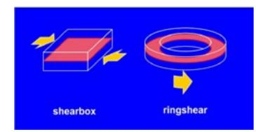
When multiple tests are performed at different normal stresses (usually three) two important parameters can be derived: apparent cohesion (c') and angle of friction ( $\varphi$ ' or phi'). Note that these parameters have dashes after their symbols: they are effective stress parameters as they are tested slow enough to be drained (even though they appear in the 'Total Stress' section of BS1377 since pore pressure is not measured).
