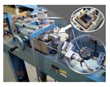
This is the most common form of shearbox test, usually performed on a 60mm square cross-section:
