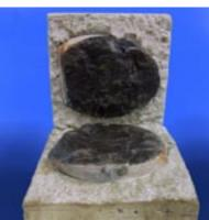
The rock specimen, wired securely so the shear plane is immobilised, is embedded either side of the shear plane in Plaster-of-Paris, grout or concrete. This allows the specimen to be
