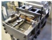
These variations can affect the shear strengths measured due to the additional restraint from a fixed load cap. At Geolabs we have UK and American style shearboxes, but have modified our American style box to permit the loading cap to be fixed or pivoting. selves, possibly giving a bit more 'bite'. An unmodified ASTM specification shearbox will not meet BS1377 requirements:
