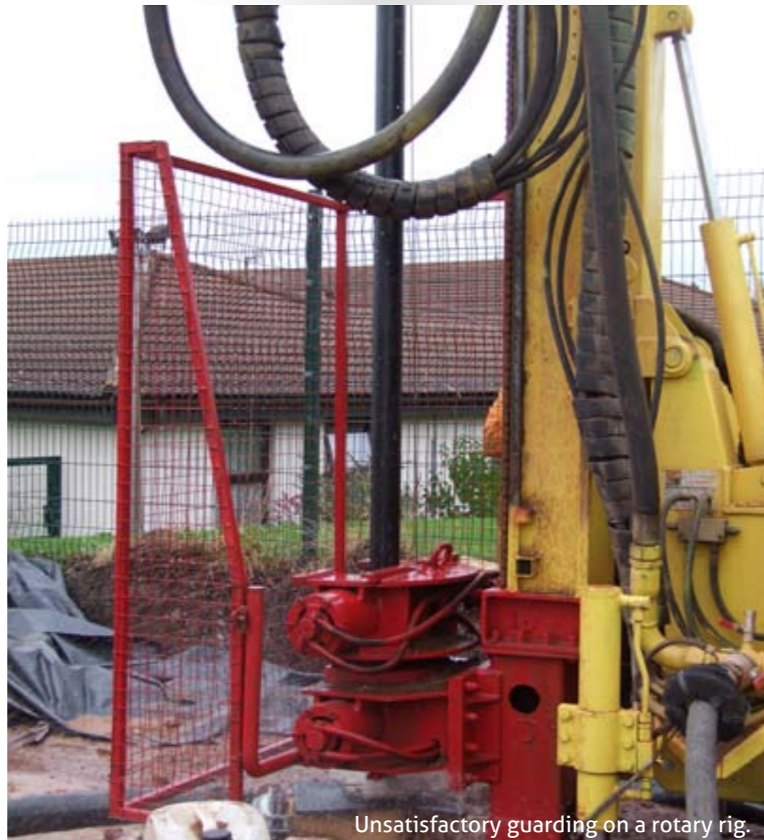
No winch guarding - does not conform to PUWER regulations.
